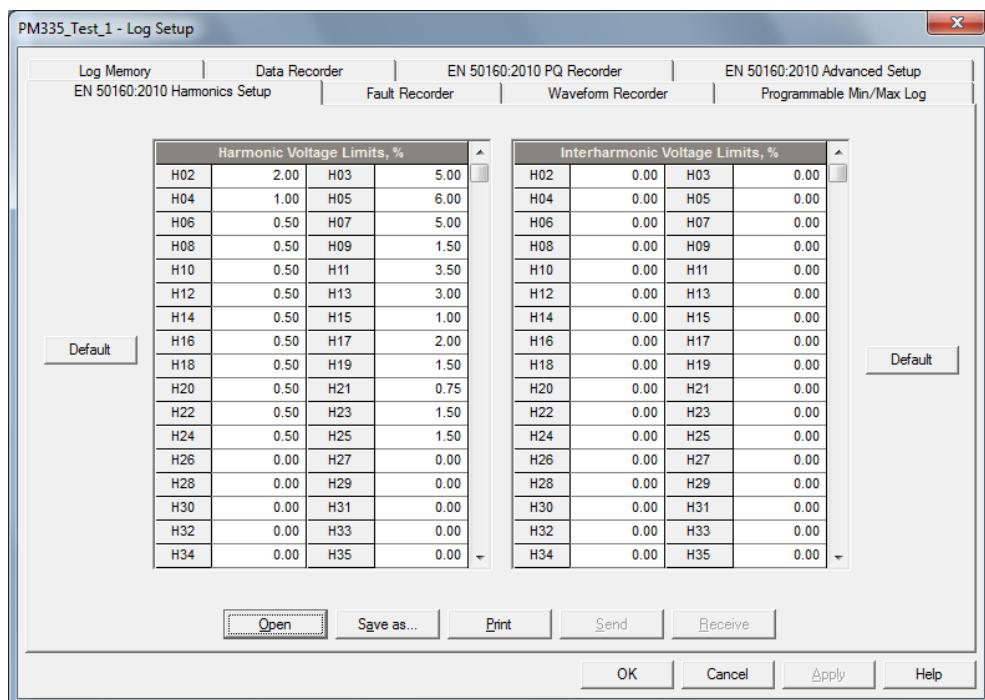
The default settings contain values of individual harmonic voltages specified by the standard for low-voltage networks. To automatically pre-set compliance limits for a medium-voltage or high-voltage network, ensure that the nominal voltage and PT ratio settings in your device's Basic Setup match the actual network characteristics, and then click on the Default button.
