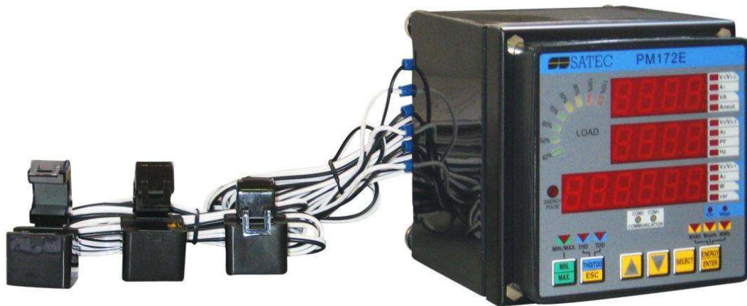
Figure 1: PM172E-HACS with 3 external split core current transformers
