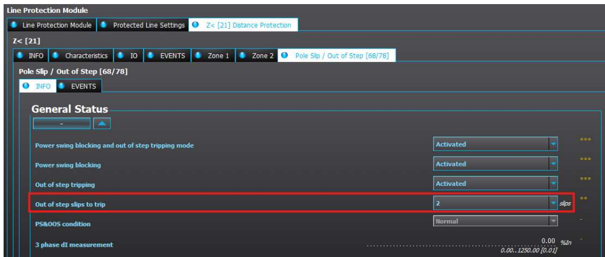
Figure 33. Out of step tripping settings. The setting range for the slips to trip setting is 1-5 slips.
