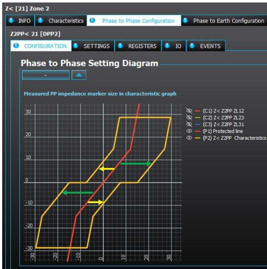
Figure 26. Non directional characteristic, "Forward-Backward" mode.
