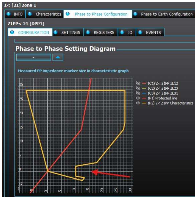
Figure 30. Load encroachment in zone characteristic.
